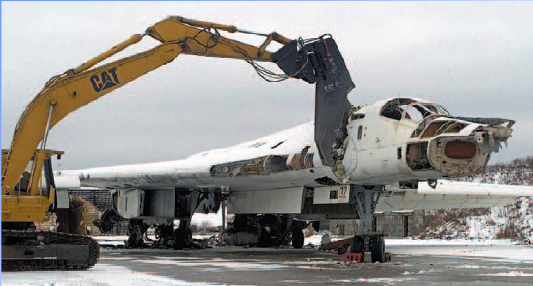
An excavator with giant scissors attached cuts off the nose of a Tu-160 strategic bomber at a Ukraine airbase on 2 February 2001. Elimination of the last Tu-160 was carried out under terms of the U.S.-Ukrainian Cooperative Threat Reduction Program.
